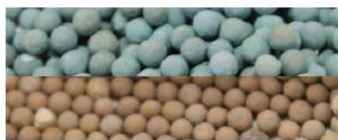
Moisture Adsorbent: Top: Full Capacity; Bottom: Depleted.
